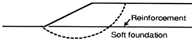
d) Basal reinforcement on soft foundations
